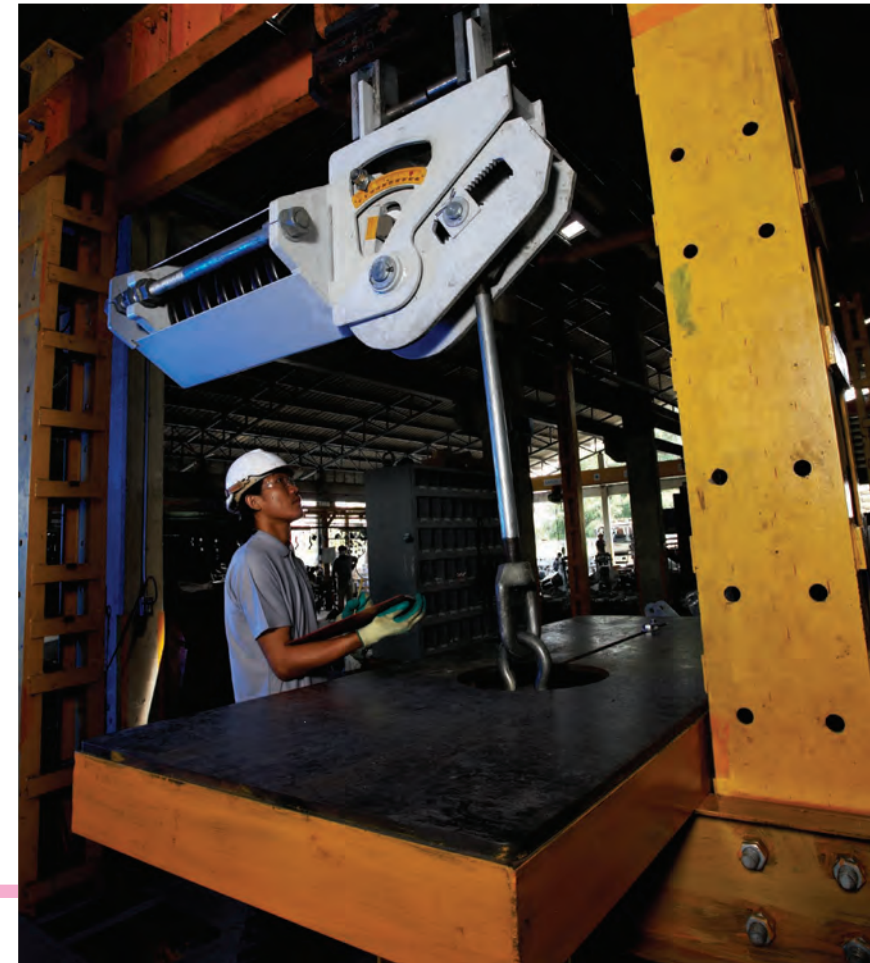
Constant Effort Support — During Load Test
