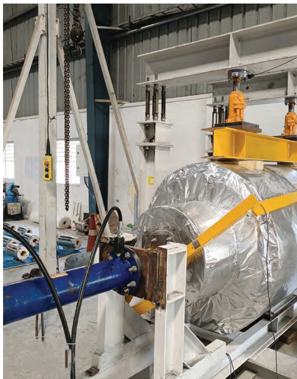
Full scale test of 30 " (750 NB) cryogenic pipe shoe at -165°C for client approval
